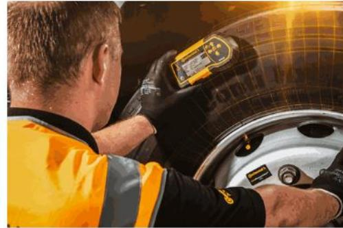
The hand-held tool is used to assign each sensor to the respective wheel position of a vehicle. The tool can also import tire data to the web portal.
